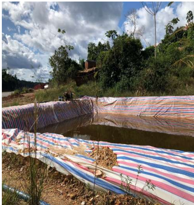
Figure 6. A barren solution pool on one of the islands in the Kwangoe area
