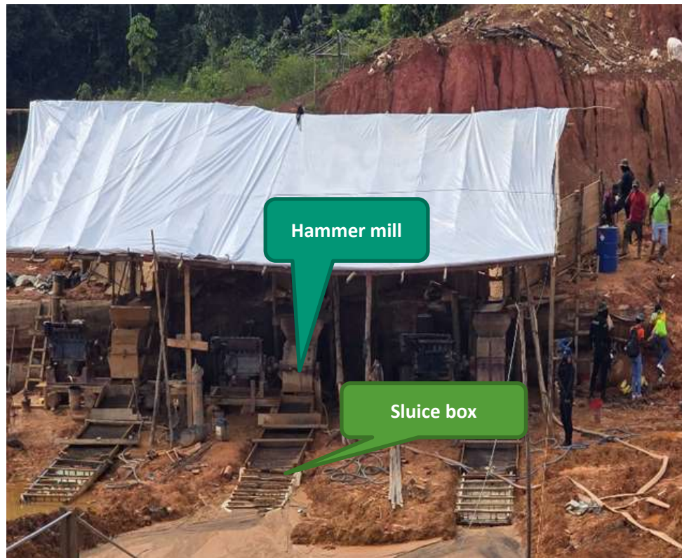
Figure 1. Hammer mill – sluice box setup (This type of setup is the most commonly used processing circuit in the ASGM sector in Suriname)
