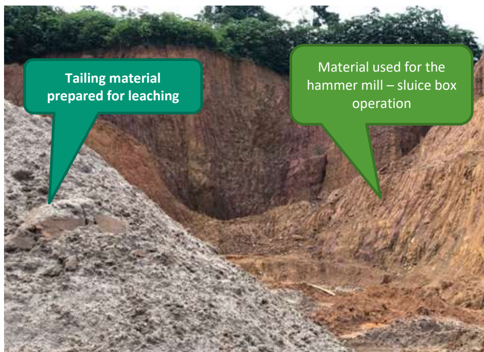
Figure 5. Prepared tailing material and raw tailings before leaching
