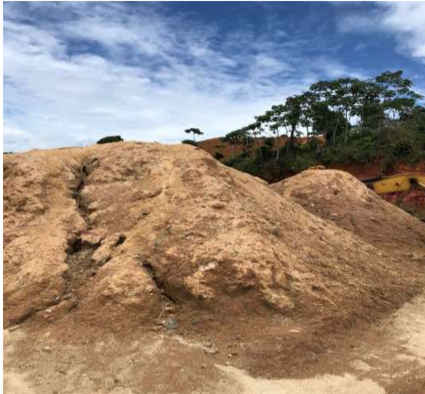
Figure 3. Material already mixed with cement and caustic soda for the leaching process
