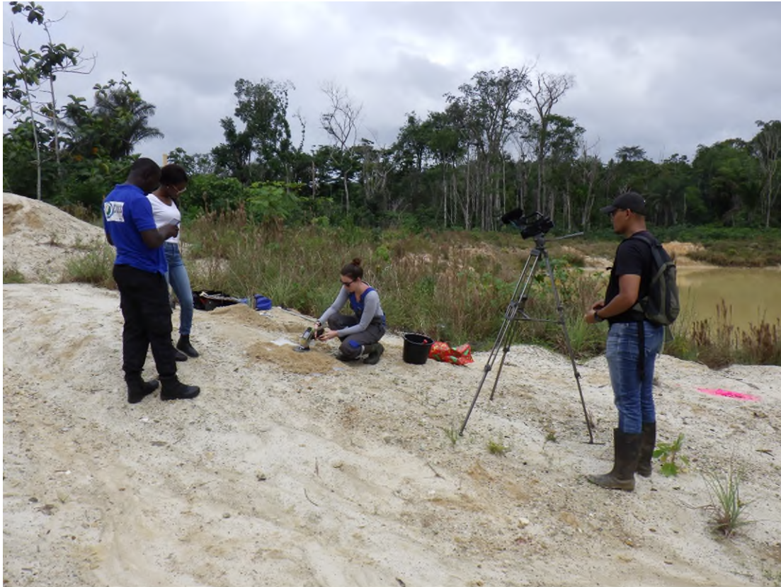
Figure 5 XRF measurements to determine the heavy metal and nutrient concentrations in the soil
